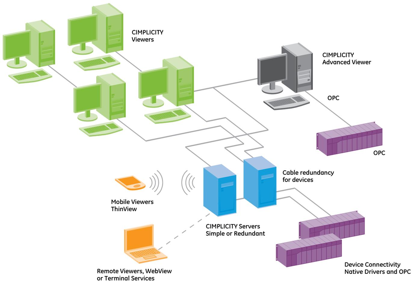
CIMPLICITY is a highly scalable solution that can run in a simple or redundant architecture with a wide variety of viewer or client options to offer flexibility when architecting your solution, providing you with more control over how and where you view your data.
