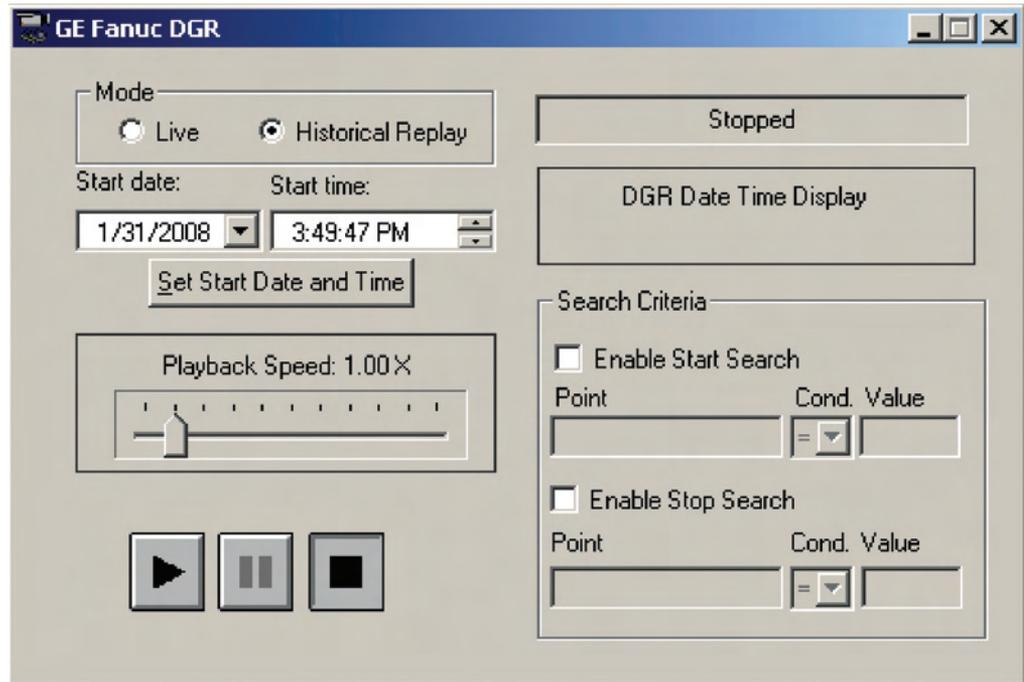
A powerful troubleshooting tool, DGR allows you to play back from a point in time, or you can have the DGR search for conditions in the data and automatically set start and stop times based on those settings to determine the cause of events.
