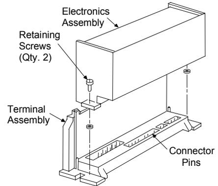
1. Unscrew the retaining screws at the top and bottom of the block.
