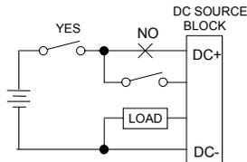
**Caution:** If circuit power is not removed at the same time as block power, the block may power up when multiple inputs are activated, even though one leg of power has been removed from the block.
