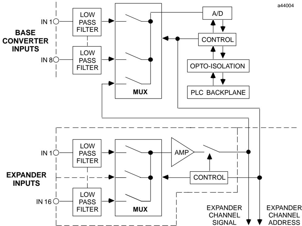
Figure 4. High Level Analog Input System Block Diagram
