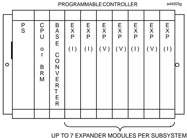
Figure 3. Example of High Level Analog Input System
