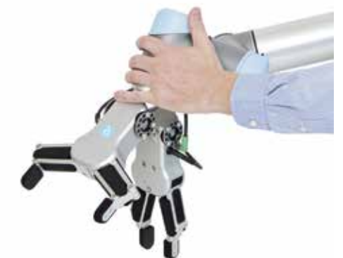
Free-Drive Mode for Manual Programming and Positioning
