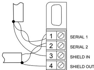
If the block is at either end of the bus, connect a terminating resistor of the appropriate type (see the *System and Communications User's Manual* for details) across its Serial 1 and Serial 2 terminals.
