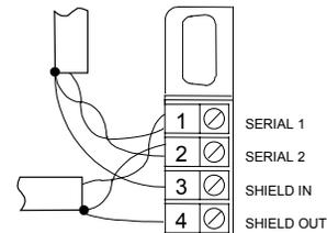
If the block is at either end of the bus, connect a terminating resistor of the appropriate type (see the *System and Communications User's Manual* for details) across its Serial 1 and Serial 2 terminals.
