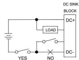
**Caution:** If circuit power is not removed at the same time as block power, the block may power up when multiple inputs are activated, even though one leg of power has been removed from the block.
