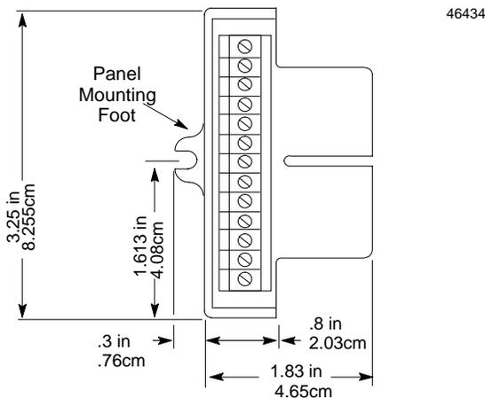
The I/O Terminal Block must be mounted on the DIN rail before installing an Auxiliary Terminal Block.
