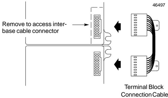
The connectors are keyed to assure proper installation. After installing the cable, be sure it is firmly seated on both connectors.
