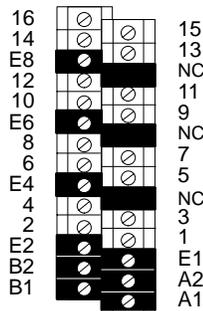
Each terminal accommodates up to one AWG #14 (2.1 mm<sup>2</sup>) or two AWG #18 (0.86mm<sup>2</sup>) through AWG #22 (.35 mm<sup>2</sup>) wires. Use copper wire rated for 90 degrees C. Recommended terminal torque is 4.5 in./lbs. The maximum current through any one terminal is 10 Amps.
