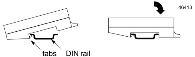
3. Tighten the DIN rail clamp screw. Recommended torque is 4 in./lb to 6 in./lb.
