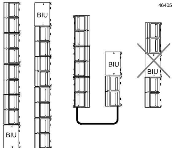
Before installing the BIU on its terminal block, install the connection cable to the next terminal block. A short connection cable, as illustrated below, is supplied with each I/O Terminal Block. Optional 21 inch (0.53 meter) cable is also available. Only one longer cable can be used per I/O station.
