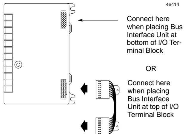
After installing the cable, be sure it is firmly seated on both connectors.
