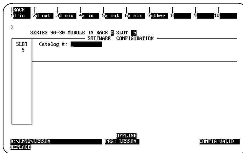
2. Press the **a in**, softkey (F4) to display a list of available analog input modules and their catalog numbers.
