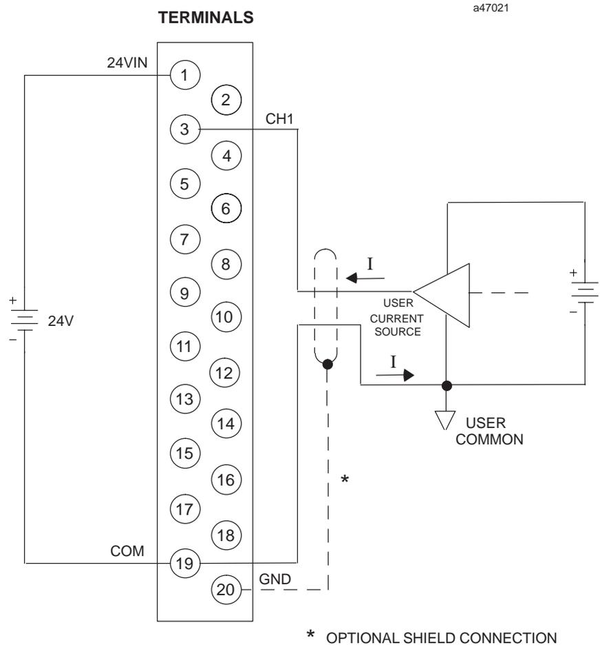
**Figure 10-17. Field Wiring - Alternate User Connections - IC693ALG223**
