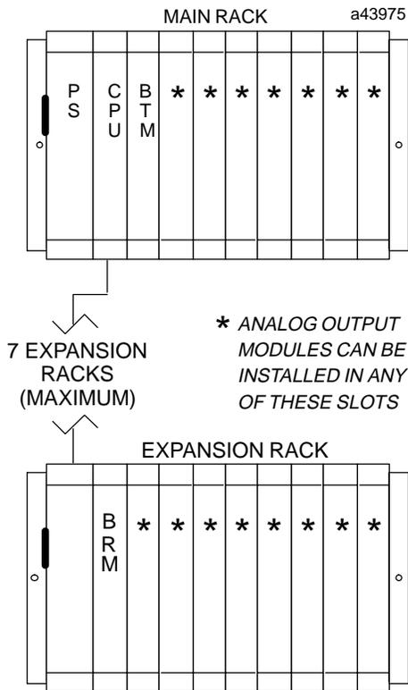
Figure 8. Example of Analog Output Module Installation
