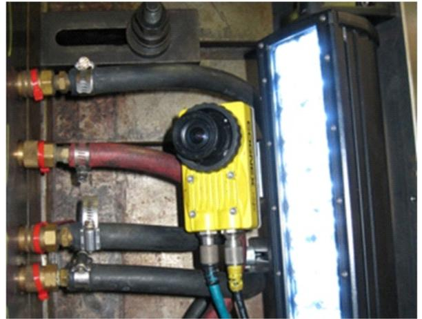
An injection molding fabricator has overcome this problem by using the Cognex In-Sight® vision system, which was trained in minutes simply by taking images of the mold in the proper condition without a part. The vision system now checks the mold for the presence of the part on every cycle, eliminating the risk of damage to the mold. The mold monitoring system has also improved quality by enabling the press to run in automatic mode, which increases cycle time consistency.
